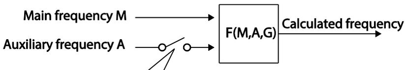
Auxiliary frequency command does not work if the multi-function terminals (In.65-71) are set to 40(disable aux. reference).
