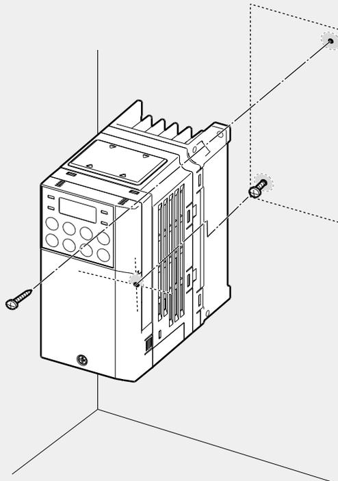
0.4kW (Single Phase) and 0.4-0.8kW (3-phase) inverters have only two mounting brackets.
