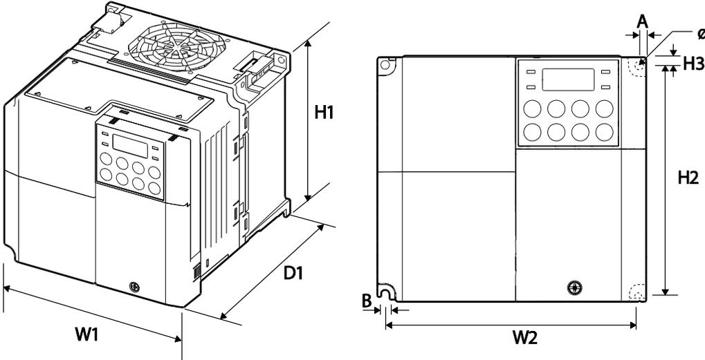
2.2kW(Single Phase 200V), 3.7-4.0kW(3-Phase 400V) EMC filter Type
