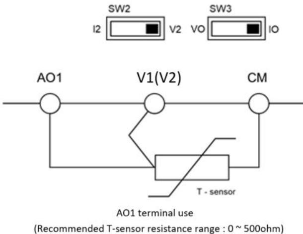
**In case of using the temperature sensor such as the PTC using a TI terminal.**
