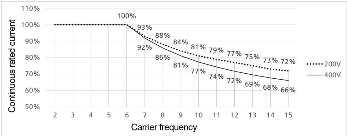
Continuous Rated Current Graph (30-75kW Heavy Duty)
