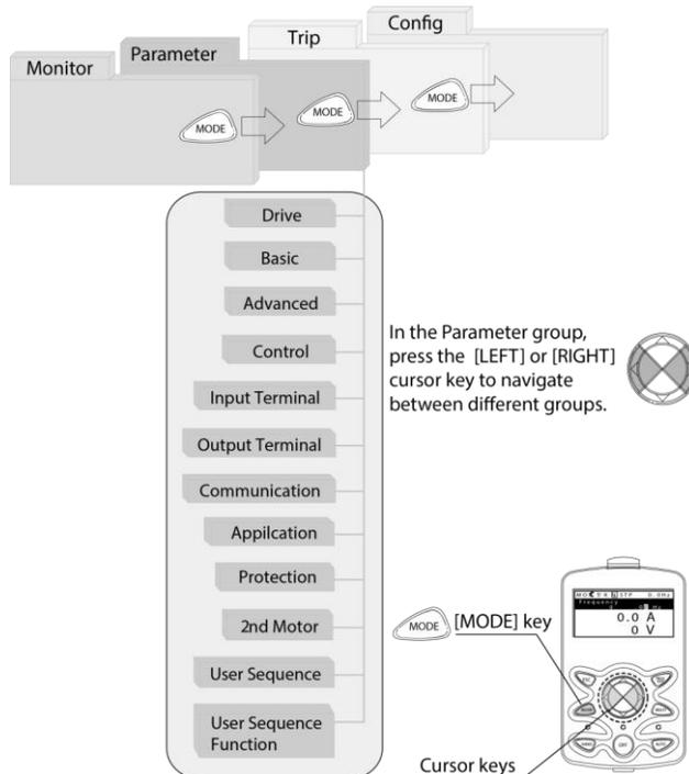
The following table lists the 5 display modes used to control the inverter functions.
