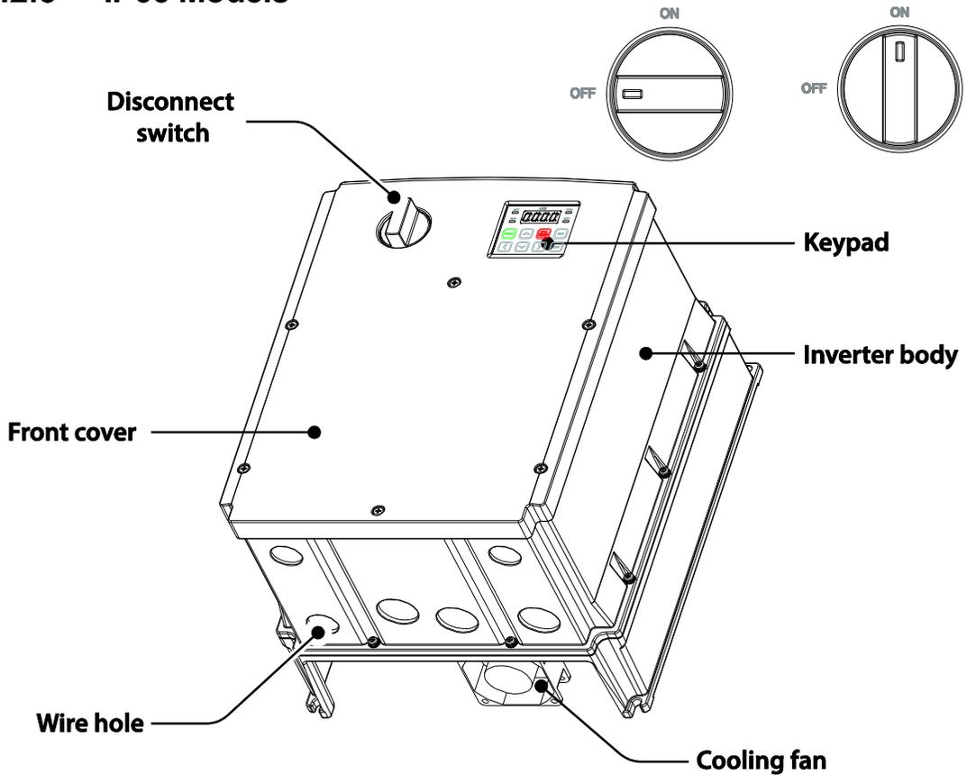
**Do not operate Disconnect Switch when motor is operating.**
